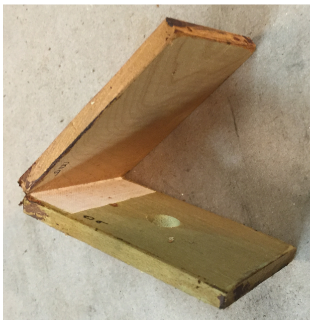
Below: A secondary with the leather cleaned off. The linen hinge, (which is also being replaced) goes from inside to outside to take the force of the pneumatic "inflating to play" rather than "deflating to play" like in the key action relay.
